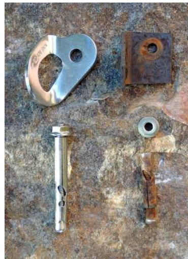
Recent bolt replacement, old and new
